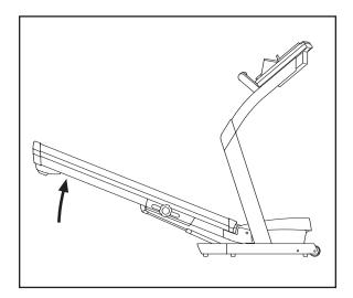
2. Move your right hand to the position shown and hold the treadmill firmly. Using your left hand, pull the latch knob to the left and hold it. Raise the treadmill until the latch pin is aligned with the hole in the housing, and insert the latch pin into the hole. **Make sure that the latch pin is fully inserted into the hole.** Note: If the adjustment knob (see page 26) hits the right upright, press on the knob.
